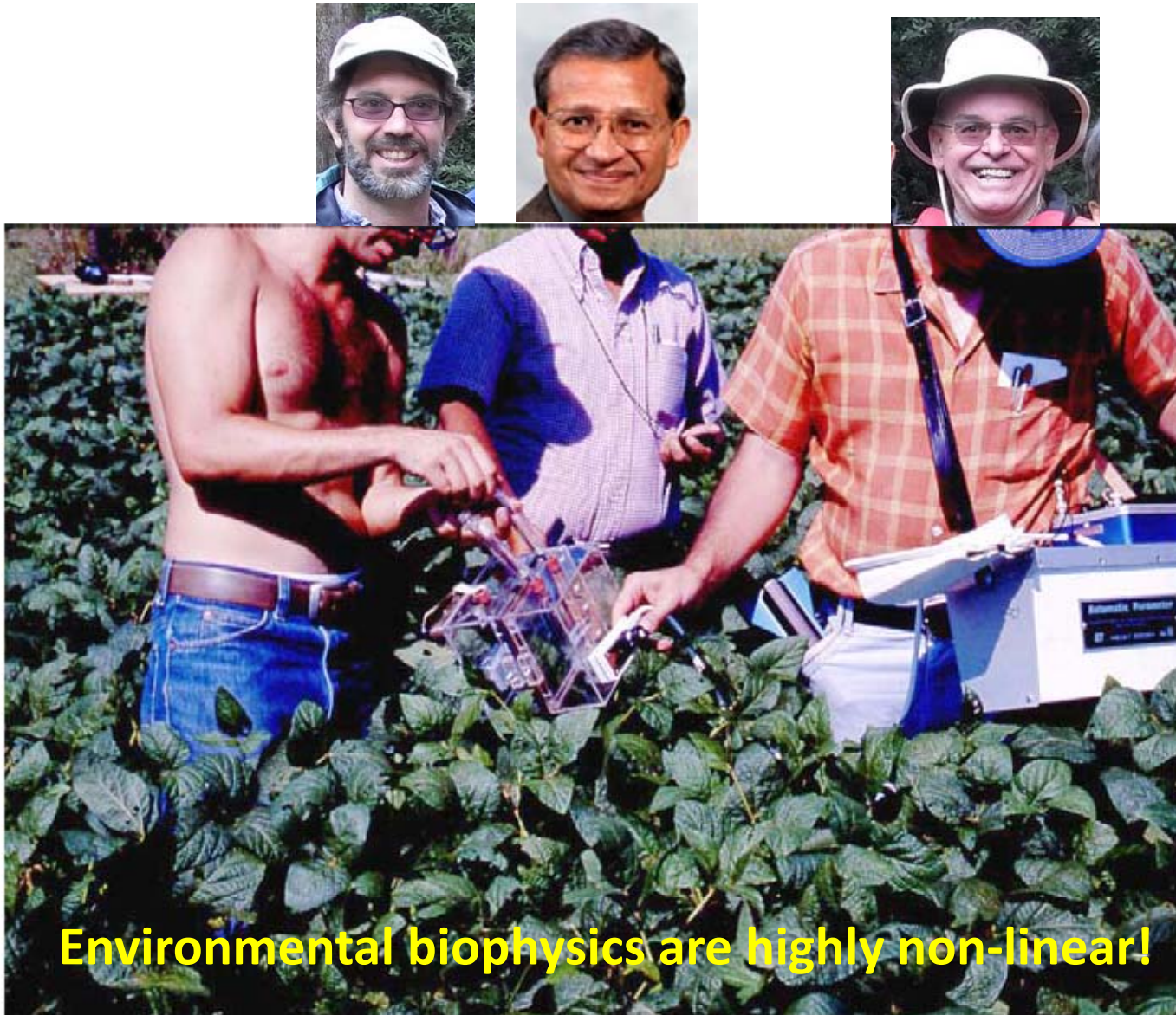
Fig. 4. John Norman (right) making “simultaneous” measurements of stomatal conductance and photosynthesis, using a Delta T porometer, and a home-made chamber with syringes.
